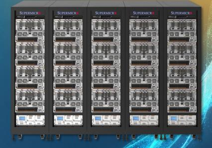
Liquid-cooled Al Rack Integrated Solutions SYS-821GE-TNHR. AS -8125GS-TNHR
