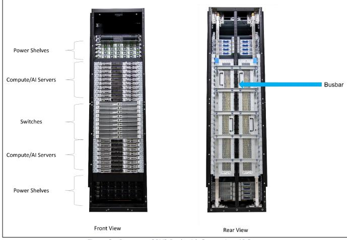
Figure 3 - Prototype ORV3 Rack with Supermicro AI Servers
