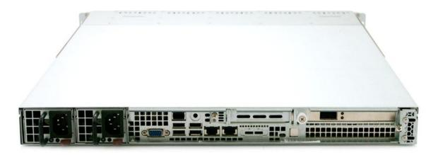
The I/O back panel of the 1027R-WC1NRT includes a VGA port, four USB 2.0 ports, two gigabit Ethernet ports, one dedicated IPMI port, an UID button and LED (both of which are located beside the PCI-E slots). The rear also houses the 700W power supply, which is composed of two separate power modules in order to provide power redundancy. This allows users to replace a failed power supply module without having to shut down the server.
