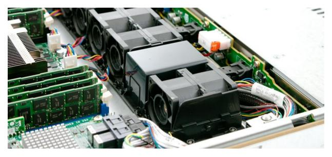
Supermicro also included their SuperCap with this server, which replaces fan module and is used for power backup for the LSI MegaRAID adapter. This puts it in a convenient position for cooling as well as servicing down the road.
