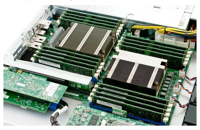
The SuperServer is intelligently laid out and compact under the hood; the X9DRW-CTF31 serverboard has 16 DIMM slots that can support up to 1024GB of ECC LRDIMM, up to 512GB of ECC RDIMM, or up to 128GB of ECC/non-ECC UDIMM DDR3-1866/1600/1333/1066/800 SDRAM.
