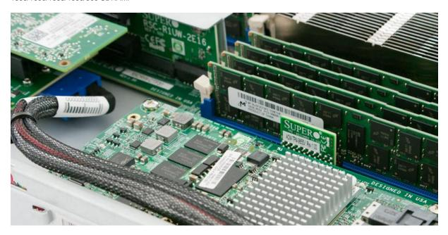
Sitting on a mezzanine card, the LSI 3108 SAS controller provides eight SAS 3.0 ports, and supports RAID levels 0, 1, 5, 6, 10, 50 and 60. In addition, a SATA controller is integrated into the chipset, providing two SATA 3.0 (6Gb/s) ports as well as two SATA 2.0 (3Gb/s) ports with RAID0, 1, 5 and 10 support. Also visible is the TPM module.
