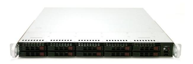
The control panel on the SC116AC2-R700WB provides important system monitoring and control information. LEDs indicate power on, network activity, and disk activity (there is also a Universal Information LED). Also present are a main power button and a UID button.
