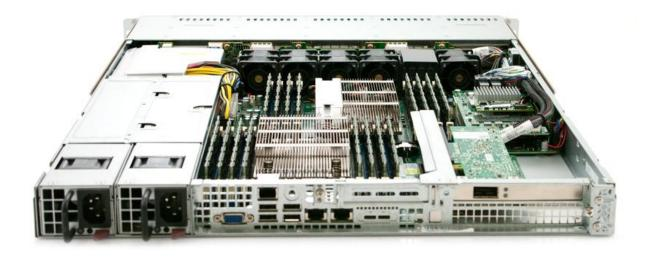
The server is easily opened after loosening one screw on the back of the chassis cover, which then slides off completely. Inside the layout is very organized, with each component quickly accessible. On the far right side of the motherboard includes an assortment of SATA ports partially obstructed by the NVMe cabling routing on that side of the chassis.
