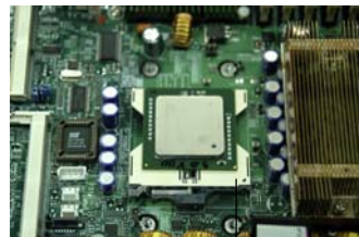
Socket lever in the locking Position
