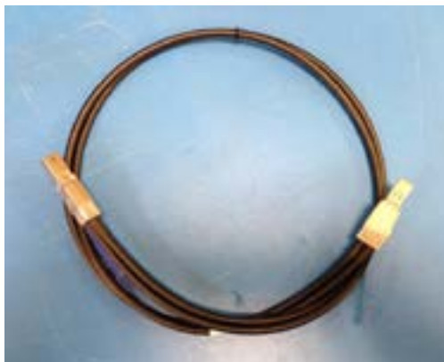
Figure A-7. External Mini-SAS HD to External Mini-SAS HD Cable
