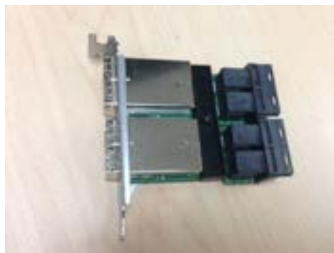
Figure A-8. Mini-SAS HD Internal to External Adapter
